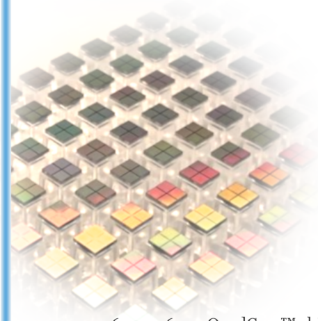
6mm x 6mm QuadCore™ chips contain 8 probes against each base in the SARS-CoV-2 genome and against common variant sequences.
